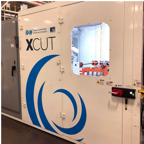
PCMC's Xcut saw features cutting-edge sensors to monitor saw blade condition.
