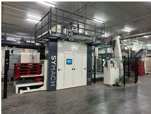
The SYMACH 3500S conventional push-type palletizer offers superior stacking and palletizing performance.
